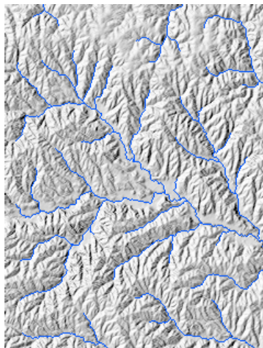
Shaded relief image of sample area with flowpaths computed by the Watershed process.
